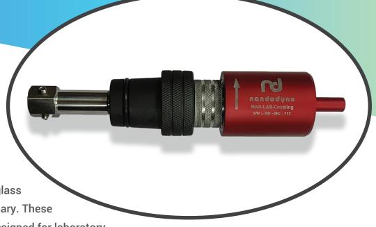
glass flasks. One end of the coupling snuggly fits on the nozzle of a glass flask while the other end can be coupled to the stirrer motor. A glass shaft with a PTFE impeller can be fitted on the bottomside. These magnetic couplings can fit various glass nozzle types such as B-34, B-29, B-24, etc. These couplings can easily handle torques of various DC Motors to stir the mass up to 200 Litre capacity.
